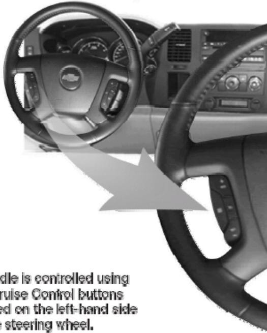
Fast Idle is controlled using the Cruise Control buttons located on the left-hand side of the steering wheel.
