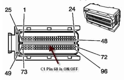
C2 pin 18 is the release and momentary switch, and C1 Pin 60 is the on/off switch.
