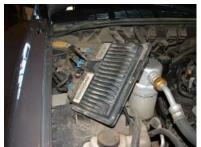
Step Five: Remove all of the blue clips from your computer. There should be 5 clips for 1996-1997 trucks and 4 clips for 1998-2000 trucks.
