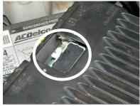
Step Ten: Fully remove the panel and there should be a knock module in the opening.
