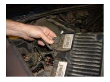
Step Six: Depress the release tab of the connector to remove all electrical connections.
