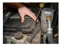
Step Three: Use a screwdriver (or tool of your preference) to aid in the release of your computer from its mounting bracket.
